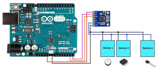
All 1-wire devices must be connected in parallel. Each device has an unique identification number, and responds only when the device is selected. Since the 1-Wire protocol is only a transport protocol, each 1-Wire slave device has intrinsic communication and protocol data characteristics. Please refer to the slave device datasheet.
