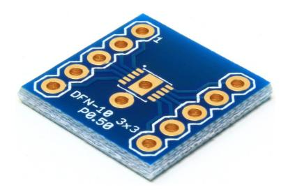
This adapter breaks out the pins of a DFN-10 component (with a body of 3mm x 3mm and 0.50mm pin pitch) into a board with 0.1" (2.54mm) spaced pins.
