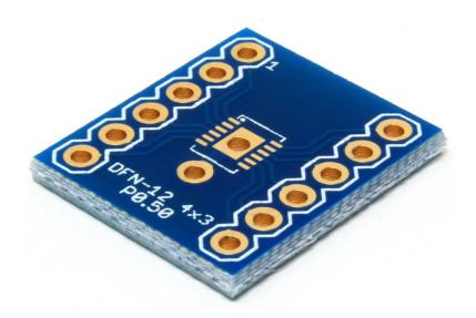
This adapter breaks out the pins of a DFN-12 component (with a body of 4mm x 3mm and 0.50mm pin pitch) into a board with 0.1" (2.54mm) spaced pins.
