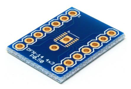
This adapter breaks out the pins of a DFN-14 component (with a body of 4mm x 3mm and 0.50mm pin pitch) into a board with 0.1" (2.54mm) spaced pins.
