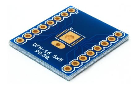
This adapter breaks out the pins of a DFN-16 component (with a body of 5mm x 5mm and 0.50mm pin pitch) into a board with 0.1" (2.54mm) spaced pins.
