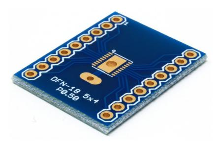
This adapter breaks out the pins of a DFN-18 component (with a body of 5mm x 4mm and 0.50mm pin pitch) into a board with 0.1" (2.54mm) spaced pins.
