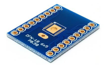
This adapter breaks out the pins of a DFN-18 component (with a body of 6mm x 5mm and 0.50mm pin pitch) into a board with 0.1" (2.54mm) spaced pins.
