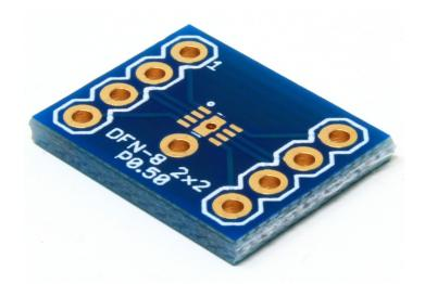
This adapter breaks out the pins of a DFN-8 component (with a body of 2mm x 2mm and 0.50mm pin pitch) into a board with 0.1" (2.54mm) spaced pins.
