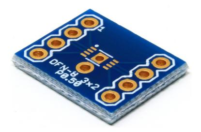
This adapter breaks out the pins of a DFN-8 component (with a body of 3mm x 2mm and 0.50mm pin pitch) into a board with 0.1" (2.54mm) spaced pins.
