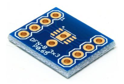
This adapter breaks out the pins of a DFN-8 component (with a body of 3mm x 3mm and 0.65mm pin pitch) into a board with 0.1" (2.54mm) spaced pins.
