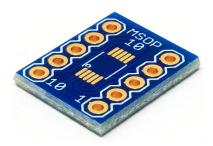
This adapter breaks out the pins of a MSOP-10 component (with a body of 3mm x 3mm and 0.50mm pin pitch) into a board with 0.1" (2.54mm) spaced pins.
