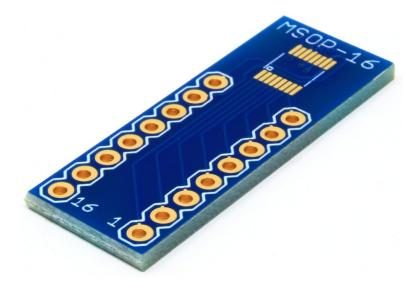
This adapter breaks out the pins of a MSOP-16 component (with a body of 4mm x 3mm and 0.50mm pin pitch) into a board with 0.1" (2.54mm) spaced pins.
