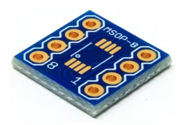
This adapter breaks out the pins of a MSOP-8 component (with a body of 3mm x 3mm and 0.65mm pin pitch) into a board with 0.1" (2.54mm) spaced pins.
