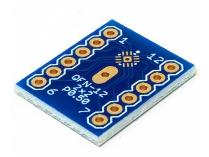
This adapter breaks out the pins of a QFN-12 component (with a body of 2mm x 2mm and 0.50mm pin pitch) into a board with 0.1" (2.54mm) spaced pins.
