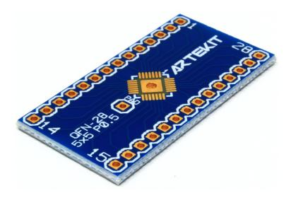
This adapter breaks out the pins of a QFN-28 component (with a body of 5mm x 5mm and 0.50mm pin pitch) into a board with 0.1" (2.54mm) spaced pins.
