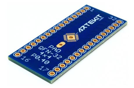
This adapter breaks out the pins of a QFN-32 component (with a body of 4mm x 4mm and 0.40mm pin pitch) into a board with 0.1" (2.54mm) spaced pins.
