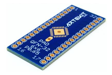
This adapter breaks out the pins of a QFN-32 component (with a body of 6mm x 6mm and 0.65mm pin pitch) into a board with 0.1" (2.54mm) spaced pins.
