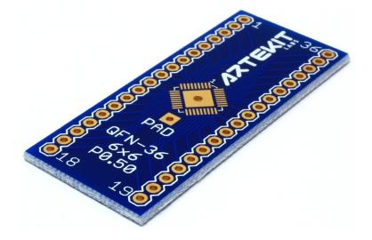
This adapter breaks out the pins of a QFN-36 component (with a body of 6mm x 6mm and 0.50mm pin pitch) into a board with 0.1" (2.54mm) spaced pins.
