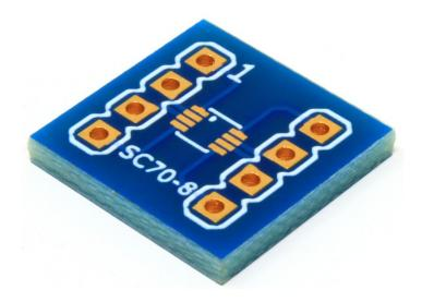
This adapter breaks out the pins of a SC70-8 component (with a body of 2mm x 1.25mm and 0.50mm pin pitch) into a board with 0.1" (2.54mm) spaced pins.
