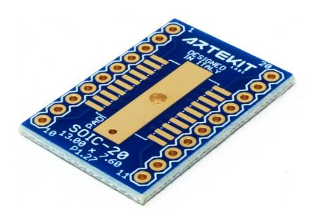
This adapter breaks out the pins of a component with SOIC-20 package (with a body of  $13\text{mm} \times 7.6\text{mm}$  and 1.27mm pin pitch) into a board with 0.1'' (2.54mm) spaced pins.
