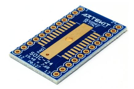
This adapter breaks out the pins of a component with SOIC-24 package (with a body of 15.4mm x 7.6mm and 1.27mm pin pitch) into a board with 0.1" (2.54mm) spaced pins.
