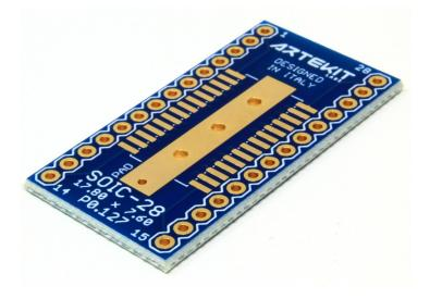
This adapter breaks out the pins of a component with SOIC-28 package (with a body of 17.8mm x 7.6mm and 1.27mm pin pitch) into a board with 0.1" (2.54mm) spaced pins.
