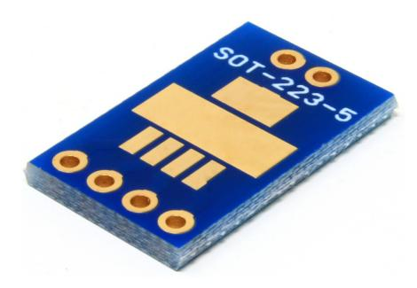
This adapter breaks out the pins of a SOT223-5 component (with 1.50mm pin pitch) into a board with 0.1" (2.54mm) spaced pins.
