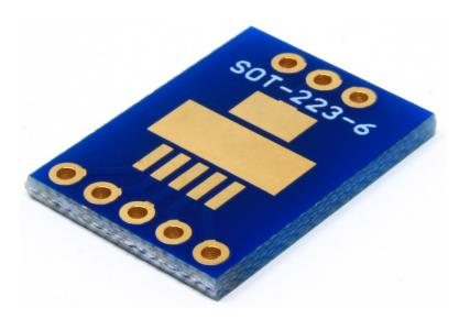
This adapter breaks out the pins of a SOT223-6 component (with 1.27mm pin pitch) into a board with 0.1" (2.54mm) spaced pins.
