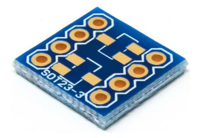
This adapter breaks out the pins of two SOT23-3 components into a board with 0.1" (2.54mm) spaced pins.
