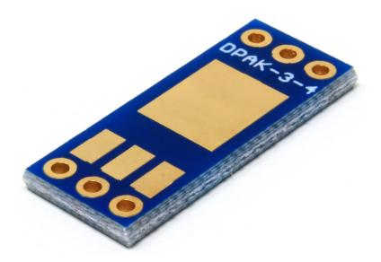
This adapter breaks out the pins of a component with TO252 package (also known as DPAK with 3 or 4 pins) into a board with 0.1" (2.54mm) spaced pins.
