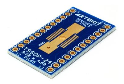
This adapter breaks out the pins of a TSSOP-24 component (with a body of 8.6mm x 4.6mm and 0.65mm pin pitch) into a board with 0.1" (2.54mm) spaced pins.
